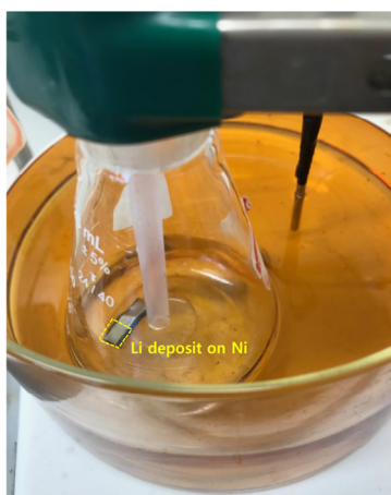
Figure S2. A picture of Li deposit on Ni substrate in an Erlenmeyer flask during nitridation.
